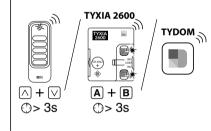
When the receiver LED has stopped flashing. The products are associated.
